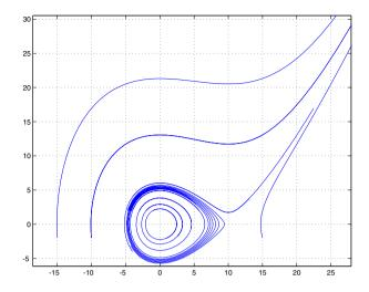
Fig. 1.2 Destabilization of the spring caused by its nonlinear stiffness
